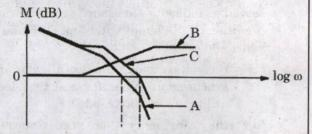
Which of the above curves is/are a compensator?
